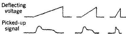
FIG. 13-28.—The type of TM obtained with a storage tube when the sweep speed is varied.
